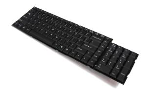
KBM-3000 is a two zone keyboard module which is specially designed for desktop/ industrial use. Its compact size and modularized mechanical design provides flexible product configuration and easy maintenance. With scissor-type key switch, it makes the touch and feel of the keycaps exceptional. We also optionally provide controller or customized codes and touchpad module as demand.
